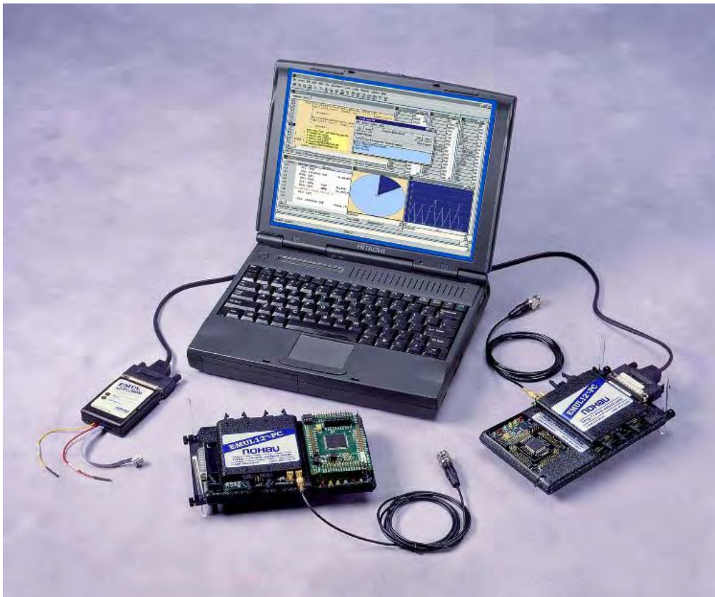
Figure 3 – various HC12 Emulators available from Nohau. On the left the BDM Emulator, on the middle the Full-Featured Emulator for the MC9S12Dxxx family, and on the right the Full-Featured emulator for the 68HC912B family. All 3 emulators are hand held, and can go anywhere your laptop can.
