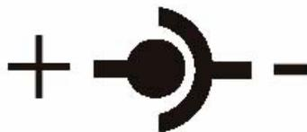
**Figure 2-5 2.0mm Power Connector**
