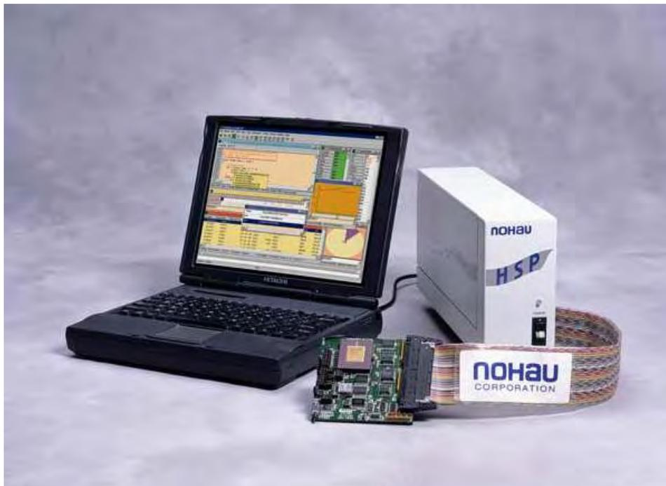
Figure 1. HSP Box Connected to a Pod Board and Laptop Computer
