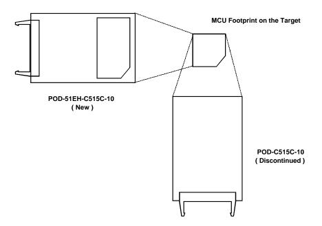
Figure 2. Pod Orientation Relative to the MCU Footprint on the Target
