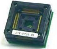
**HC12 D 112-pin to 80-pin adapter** This is a converter adapter made by Motorola, part # SC1200027-N. This adapter is used to convert a 112-pin adapter to an 80-pin package for the D60, DA128, DA128A, DG128, or DG128A emulator. This adapter is used with the ES/000-2177/78/79 (NQ) adapter or the ES/000-4534 (TQ) adapter (not included, refer to page 48 for a description).
