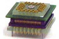
**HC12 B Winslow 80-pin QFP to PGA adapter** A Winslow 80-pin QFP to PGA adapter. This adapter is an unpopulated CPU module, that can be used with the EMUL12-B/128-16. Solder a 68HC912B32, 68HC912BC32, 68HC912BE32 or a 68HC912BD32 CPU on this adapter in order to use it as a CPU module.
