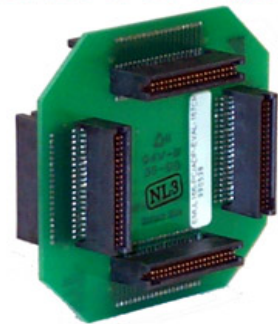
This adapter is used to connect the EMULST10 Emulator to the PHYTEC ST10 Evaluation Boards
