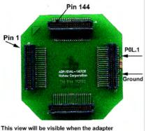
This view will be visible when the adapter is connected to the target. The emulator plugs into this side. Figure 8
