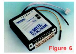
A BDM emulator does not have a trace memory, triggers or emulation memory. A BDM emulator is sometimes used in conjunction with a full emulator. It can program FLASH and EEPROM into the HC12 controller in your target system.
