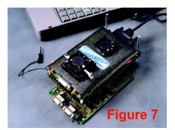
installed in the final target ready to be activated at any time for debugging. This is useful for test and repair purposes. Figure 7 is the Nohau EMUL-ST10-PC emulator connected to the Phytec C167CR evaluation board. Evaluation boards are an economical and practical method of shortening your product development time. It is also a useful reference design.
